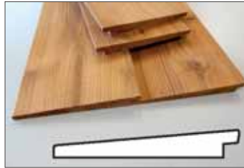
TWS21185 Thermosiding rabat 21 x 185 mm geschaafd, nuttige breedte 17.5 cm
